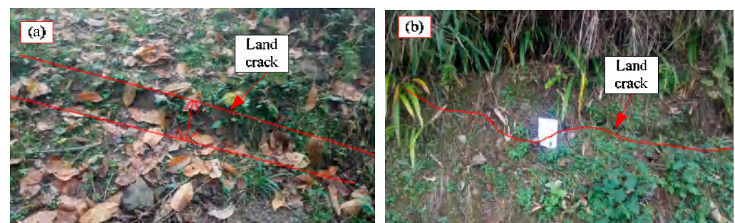
Figure 3. Cracks induced by landslide: (a) Cracks in rear edge of landslide, (b) Cracks in front edge of landslide.
