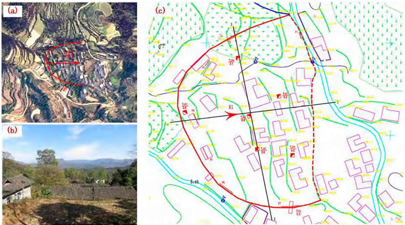
Figure 1. Distribution of landslide and the threatened area: (a) remote sensing image, (b) threatened building, (c) topographic of the landslide area.
